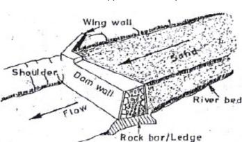
required for their construction is still high, and to involve local populations will involve training if new to the concept. Figure 16: Diagram of Sand Dam Photo: Practical Action
